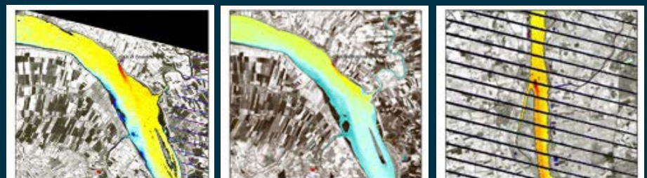
Figure 3: Examples of Landsat images showing anomalies in temperature caused by cooling water from power plants (left and right: Landsat-7, middle: Landsat-8). Shown are power plants at the Elbe River (left and middle) and the Weser River in Germany. (Brockmann Consult service; image data: Landsat ©USGS)
